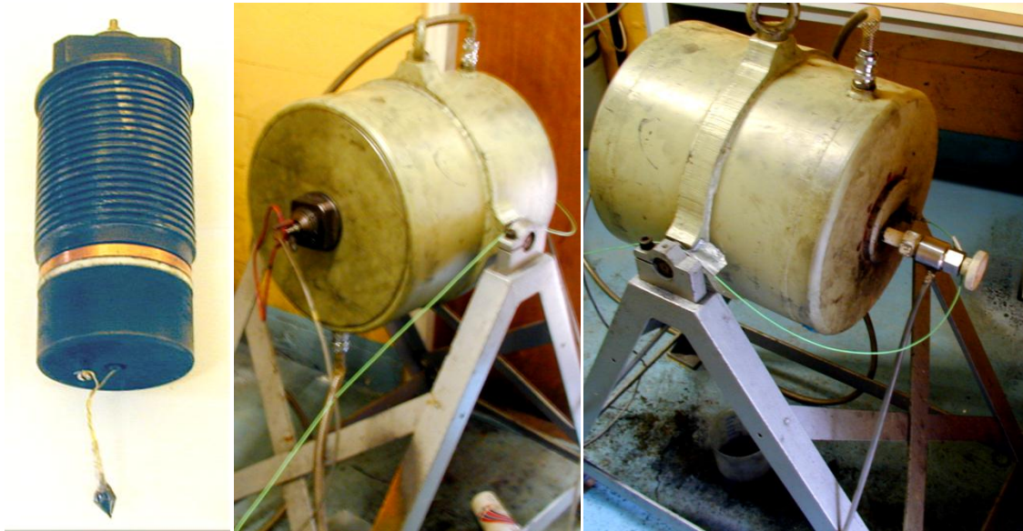
Figure 2.1 The left picture shows the igniter unit with 1g black powder and the next two pictures show the 700 cm 3 Closed Vessel.
