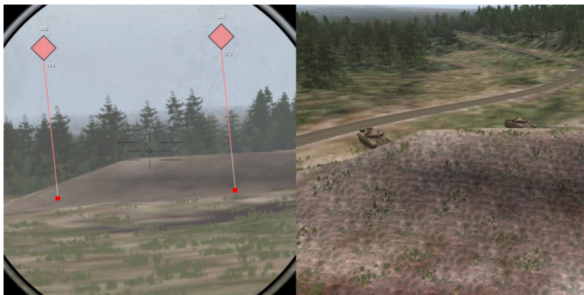
Figure 4.7 AR objects that are positioned on the other side of a hill are visualized with red dots and partially white lines.
