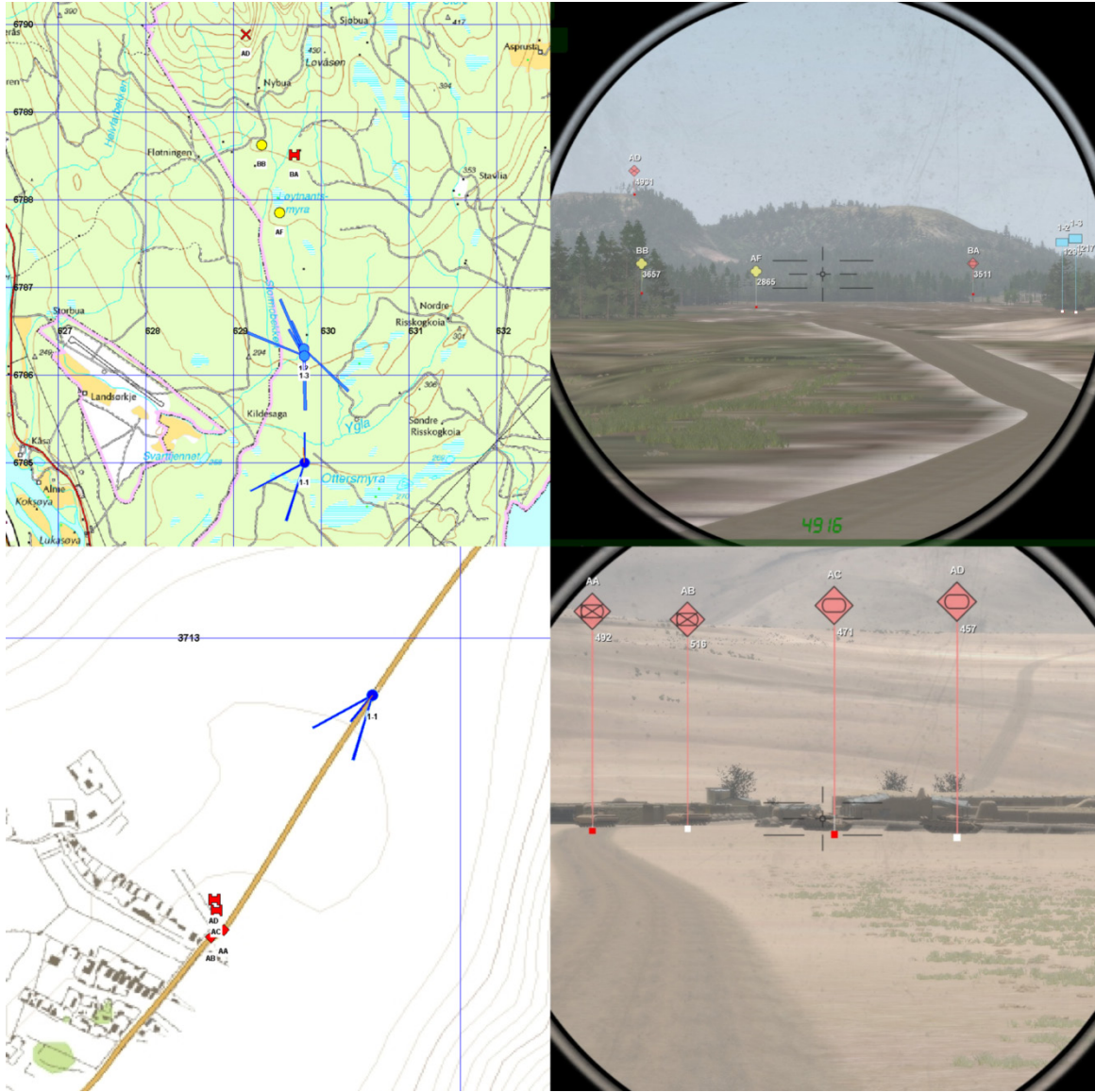
Figure 4.4 Two situations with observations on the BMS screen (to the left) and through the vehicle commander’s sight with the AR system (to the right).
