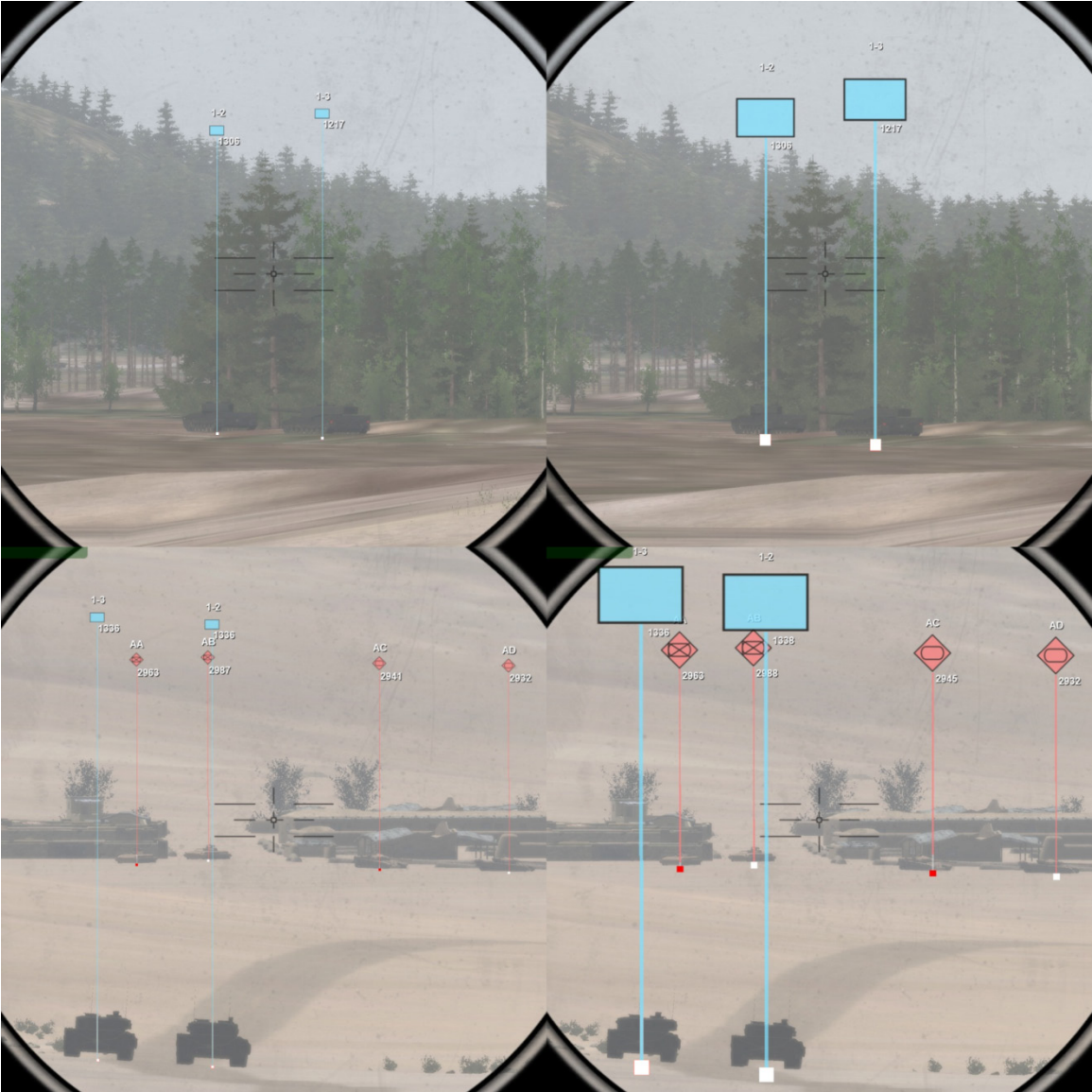
Figure 4.6 AR objects with scaling according to the distance from the vehicle turned off (to the left) and turned on (to the right).
