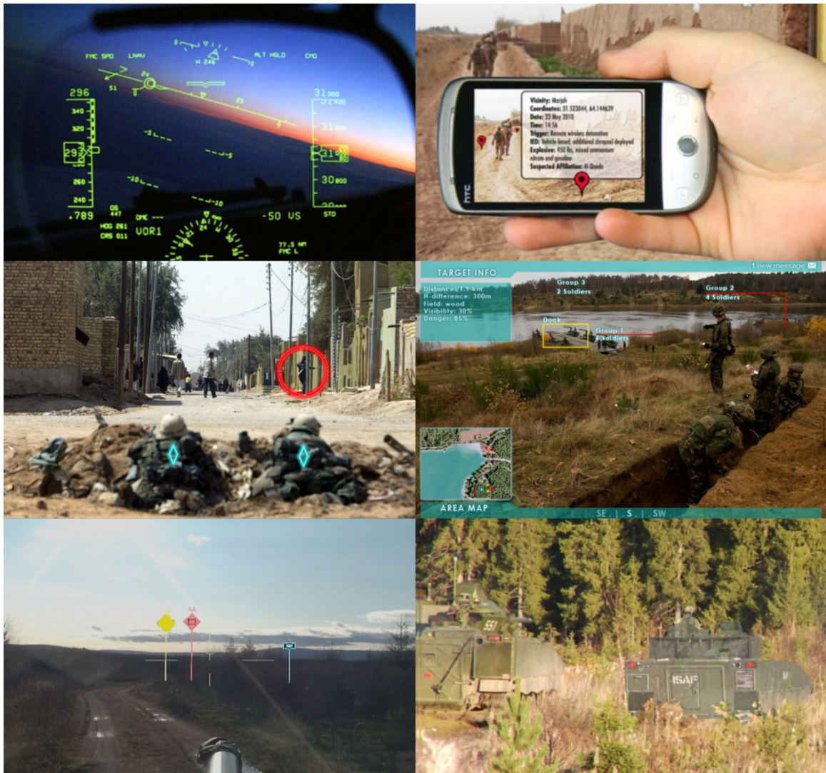
Figure 2.3 Examples of military applications of AR: HUD in aircraft, IED Threat Locator [7], ground soldier systems (Microvision and Contactum), combat vehicle system, and exercises with real and virtual units.
