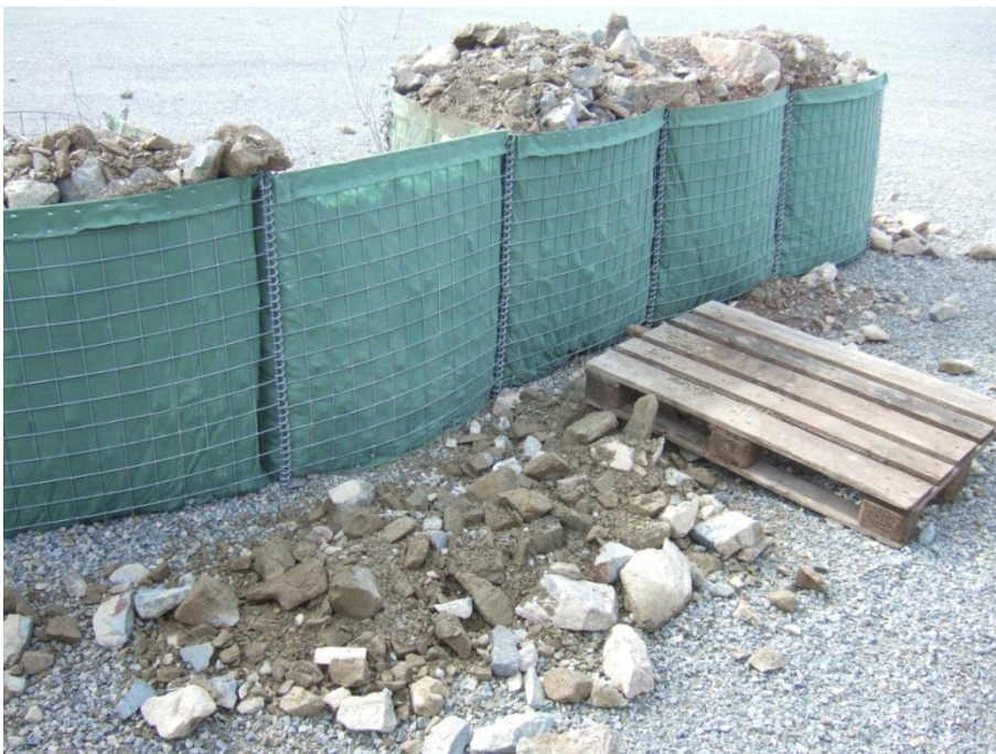
Figure 2.19 Back side of MIL 3 wall with crushed rock after detonation of 7.5 kg TNT (test 1.9)
