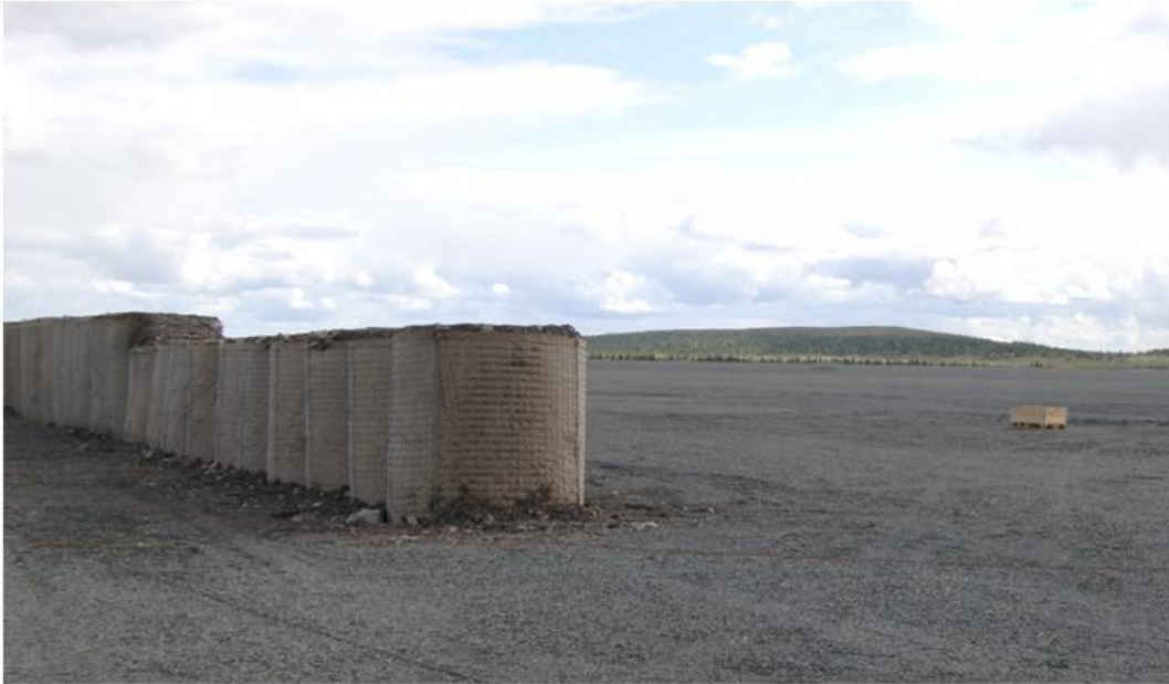
Figure 2.31 400 kg TNT 20 m in front of a buried and an unburied MIL 10 wall (test 2.1)
