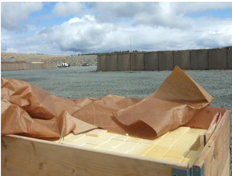
Figure 2.32 400 kg TNT charge
