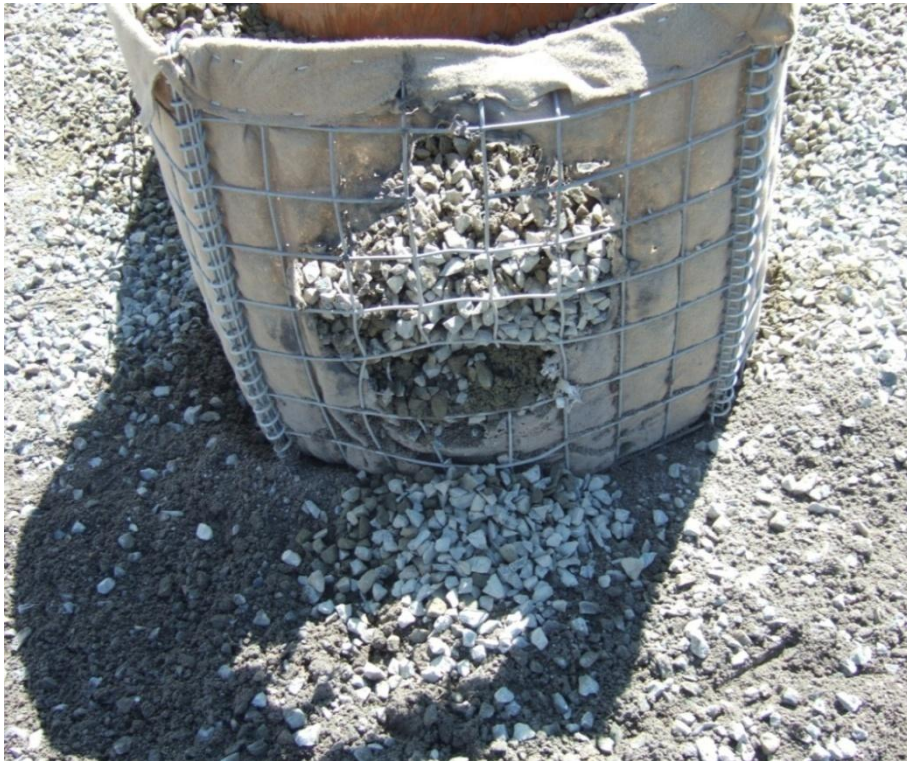
Figure 2.56 Front side of MIL 2 filled with gravel after detonation of a 340 g shaped charge
