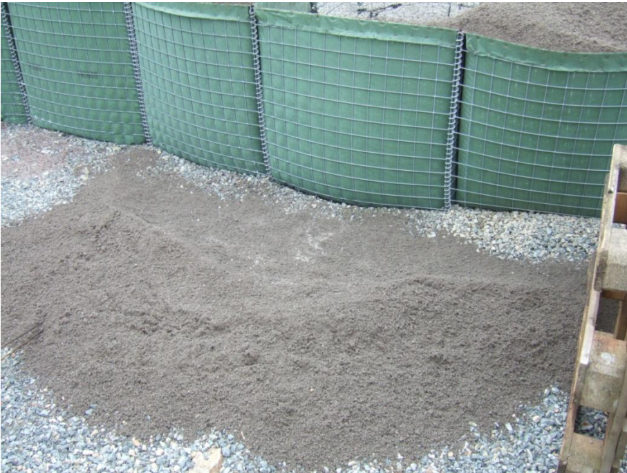
Figure 2.11 Back side of MIL 3 wall with sand after detonation of 7.5 kg TNT (test 1.2)
