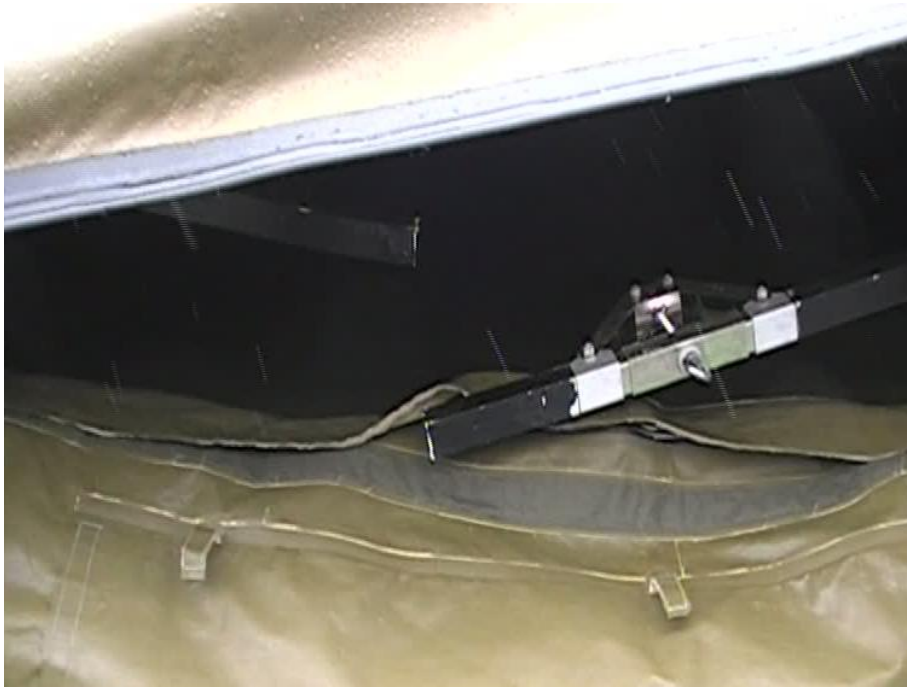
Figure 2.30 Distance rod of NM 240 tent after detonation of 7.5 kg TNT at the opposite side of a MIL 3 wall with crushed rock (test 1.4)
