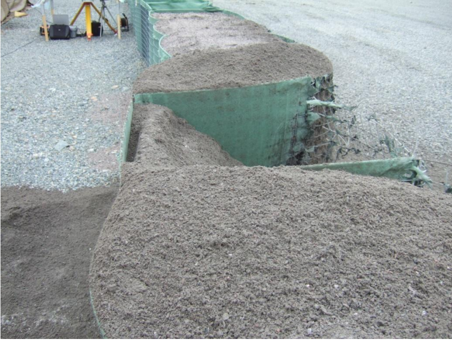
Figure 2.10 MIL 3 wall with sand after detonation of 7.5 kg TNT (test 1.2)
