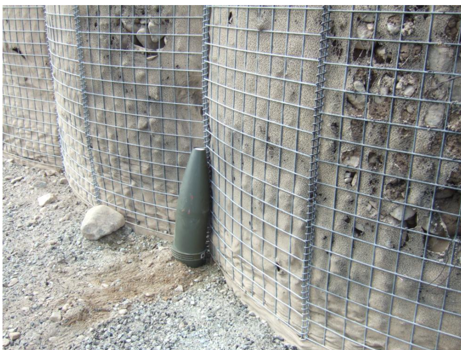
Figure 2.7 Setup of test 1.14 with a 155 shell at a MIL 10 wall with local soil
