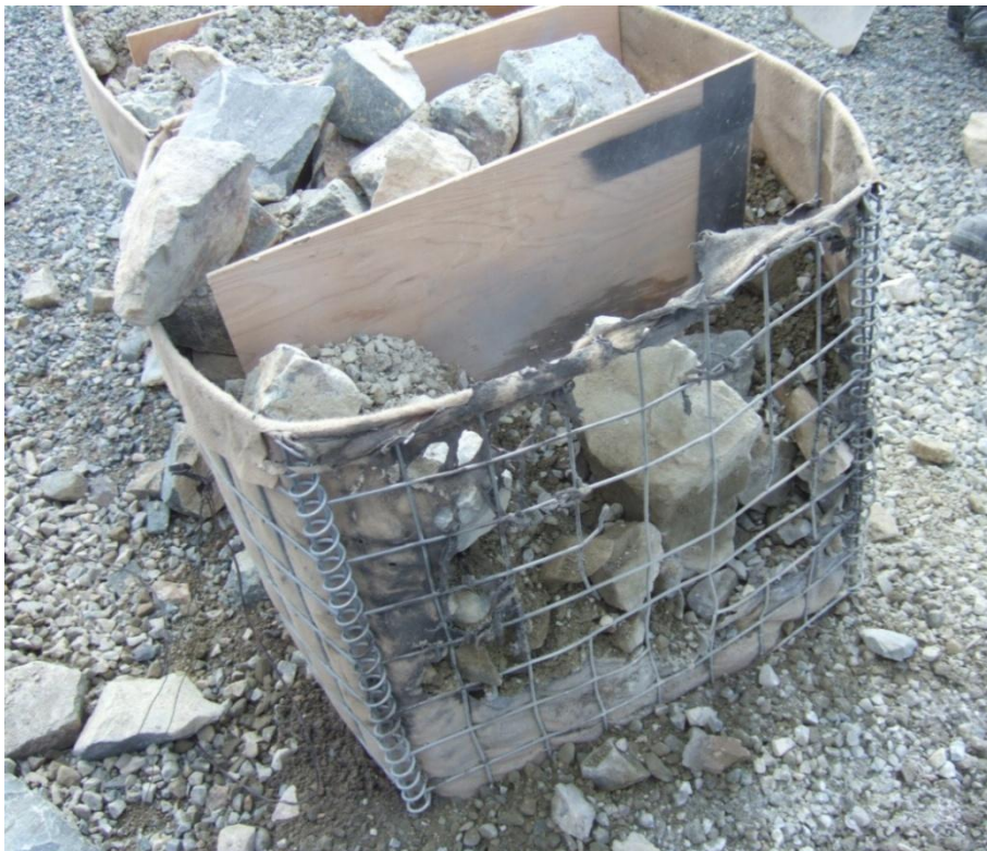
Figure 2.57 Front side of MIL 2 filled with crushed rock after detonation of a 340 g shaped charge
