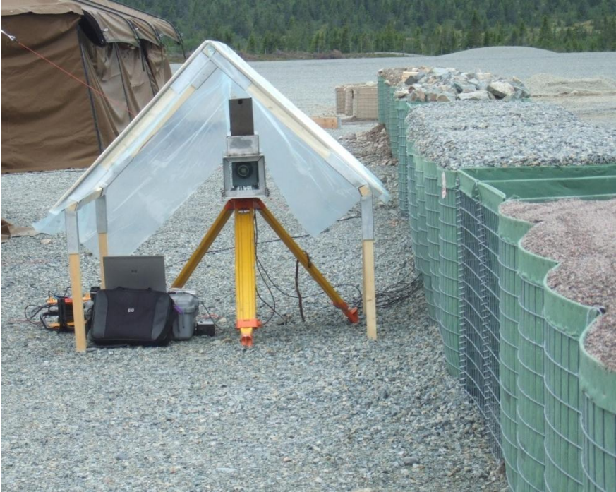
Figure 2.2 High-speed video camera in test 1.1
