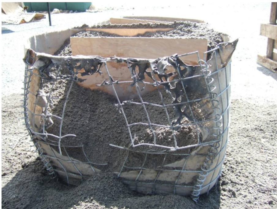
Figure 2.55 Front side of MIL 2 filled with sand after detonation of a 340 g shaped charge
