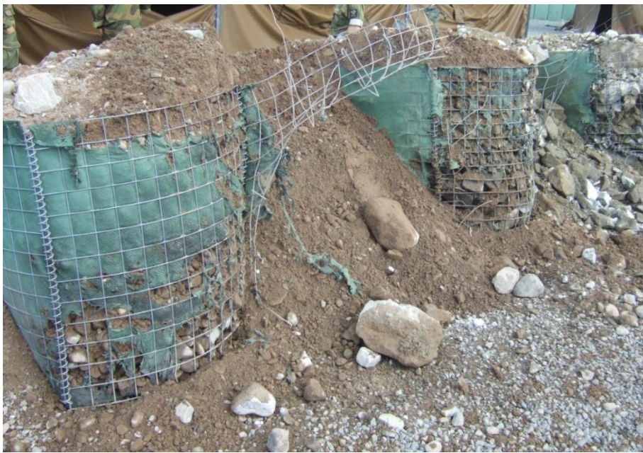
Figure 2.21 Front side of MIL 3 wall with local soil after detonation of 3.5 kg TNT (test 1.10)
