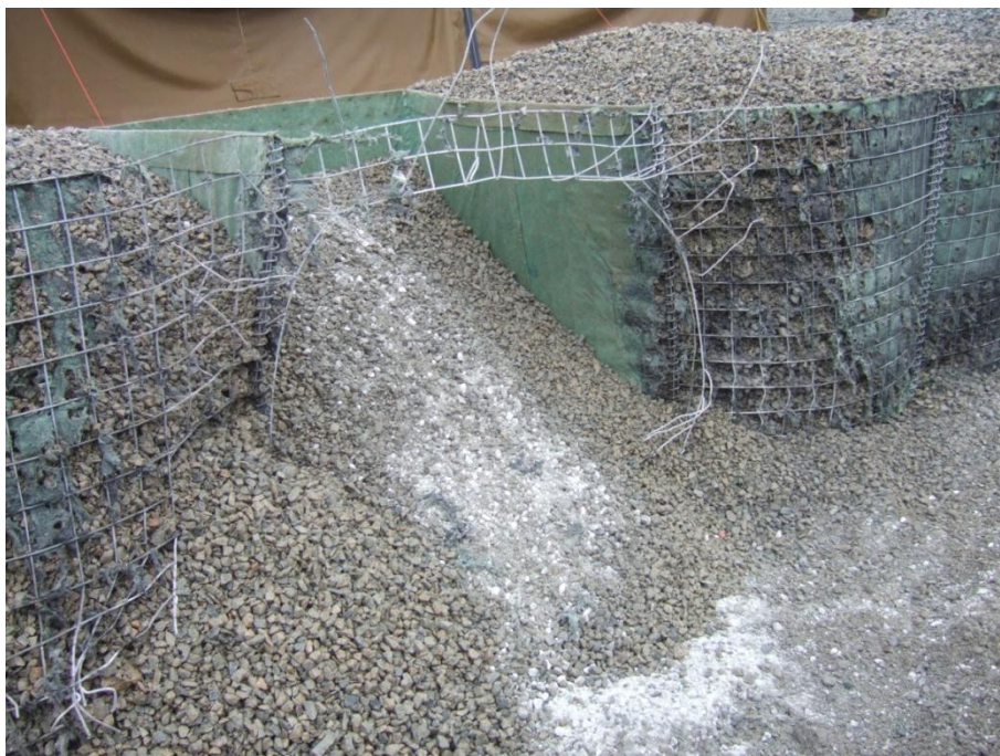
Figure 2.14 Front side of MIL 3 wall with gravel after detonation of 7.5 kg TNT (test 1.4)
