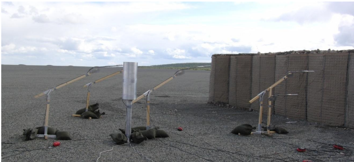
Figure 2.35 Pressure transducers behind the wall in test 2.1
