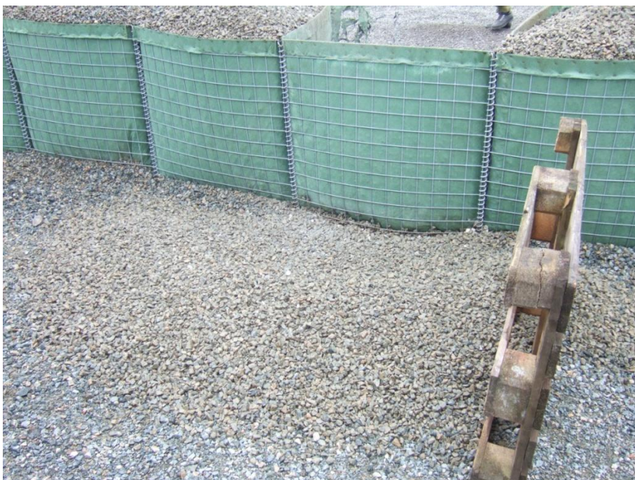
Figure 2.13 Back side of MIL 3 wall with gravel after detonation of 3.5 kg TNT (test 1.3)
