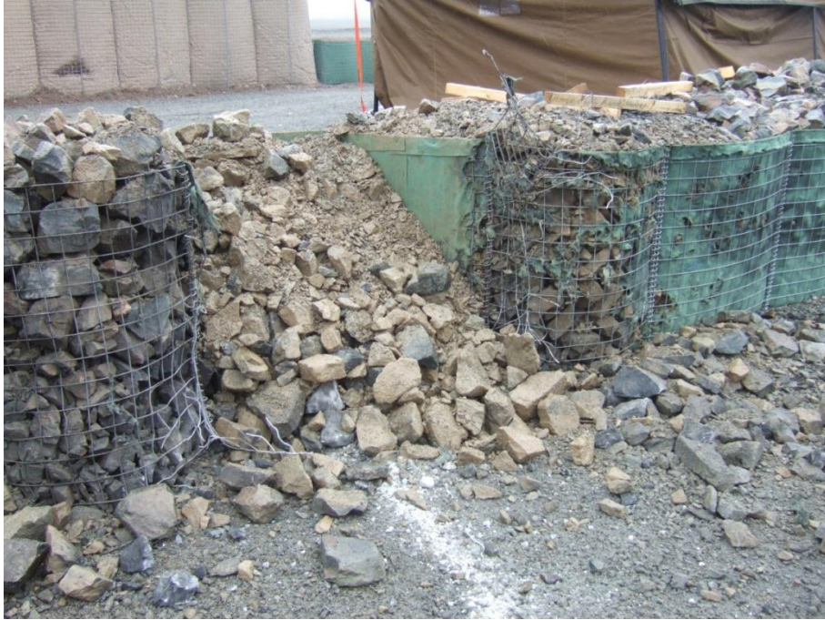
Figure 2.16 Front side of MIL 3 wall with crushed rock after detonation of 3.5 kg TNT (test 1.6)
