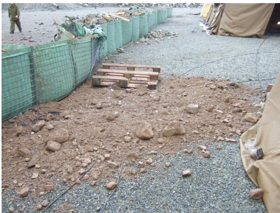
Figure 2.23 Back side of MIL 3 wall with local soil after detonation of 7.5 kg TNT (test 1.7)
