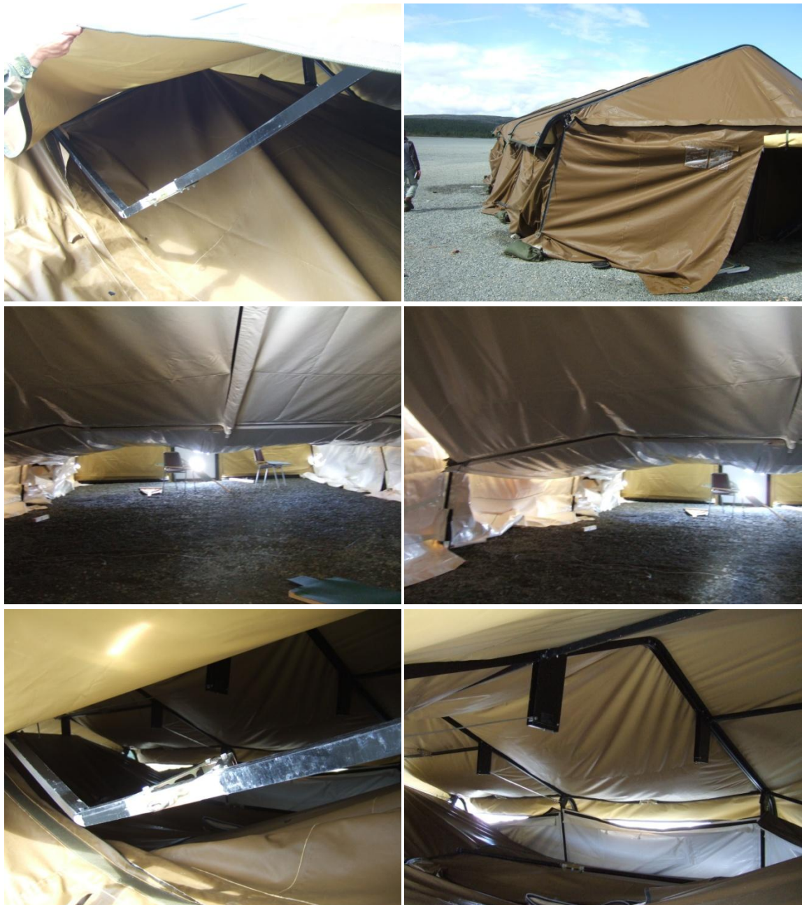
Figure 2.40 NM 240 tent after detonation of 400 kg TNT in test 2.1 about 70 m away
