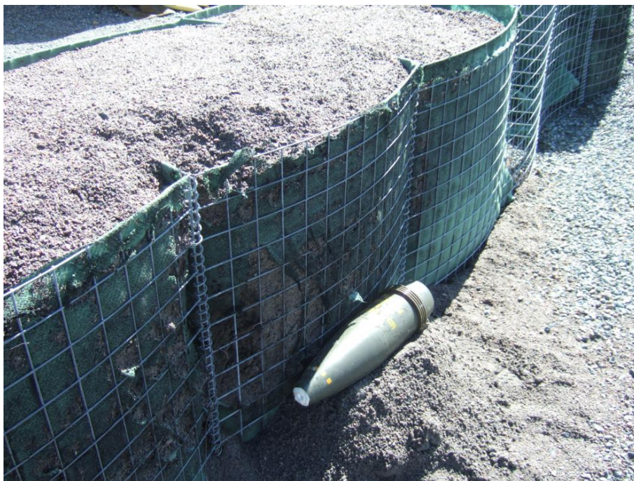
Figure 2.6 Setup of test 1.11 with a 155 shell at a MIL 3 wall with sand
