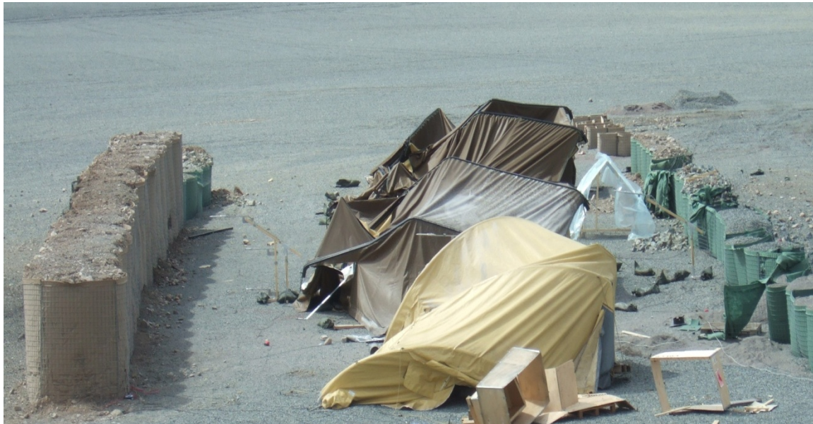
Figure 2.41 Tents after detonation of 400 kg TNT in test 2.2
