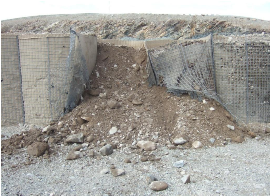
Figure 2.28 Front side of MIL 10 wall with local soil after detonation of a 155 mm grenade (test 1.14)
