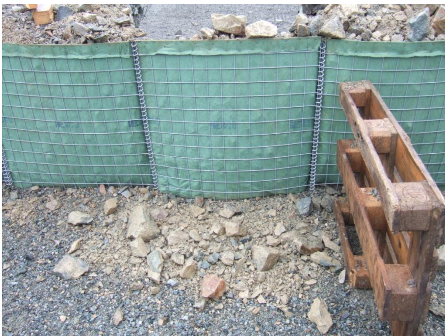
Figure 2.17 Back side of MIL 3 wall with crushed rock after detonation of 3.5 kg TNT (test 1.6)
