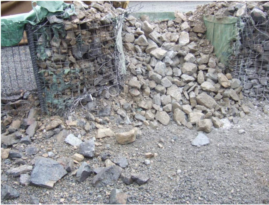
Figure 2.18 Front side of MIL 3 wall with crushed rock after detonation of 7.5 kg TNT (test 1.5)
