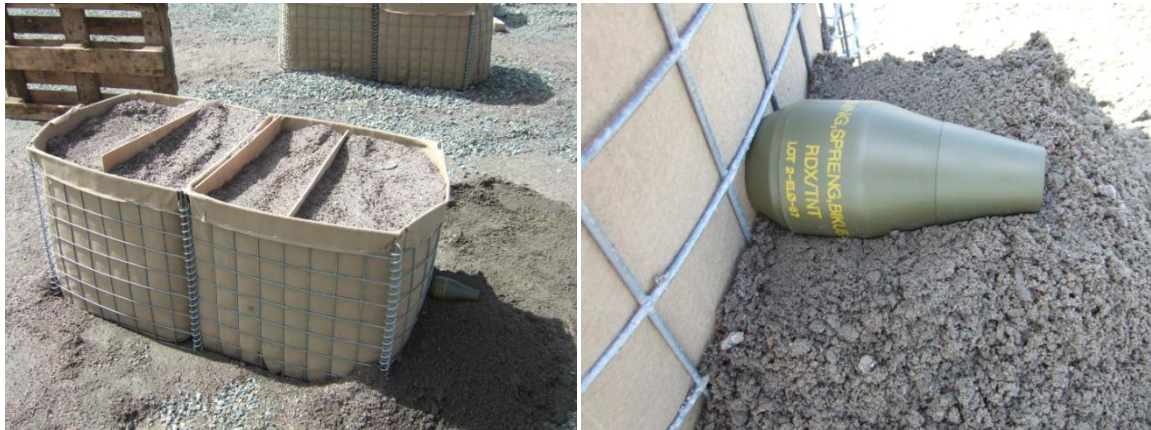
Figure 2.54 Setup of the test with a 340 g shaped charge against MIL 2 with sand
