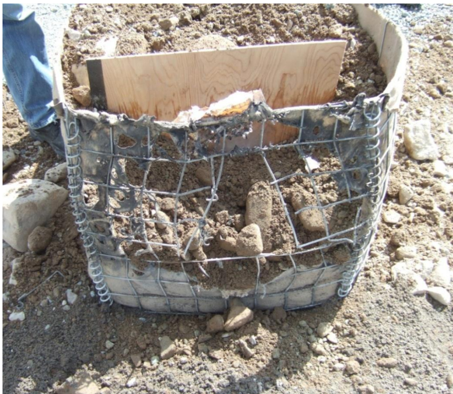
Figure 2.58 Front side of MIL 2 filled with local soil after detonation of a 340 g shaped charge
