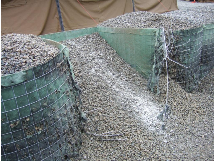
Figure 2.12 Front side of MIL 3 wall with gravel after detonation of 3.5 kg TNT (test 1.3)
