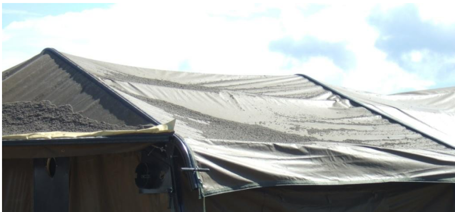
Figure 2.25 Roof of NM 240 tent after detonation of a 155 mm grenade (test 1.11) at the opposite side of a MIL 3 wall with sand
