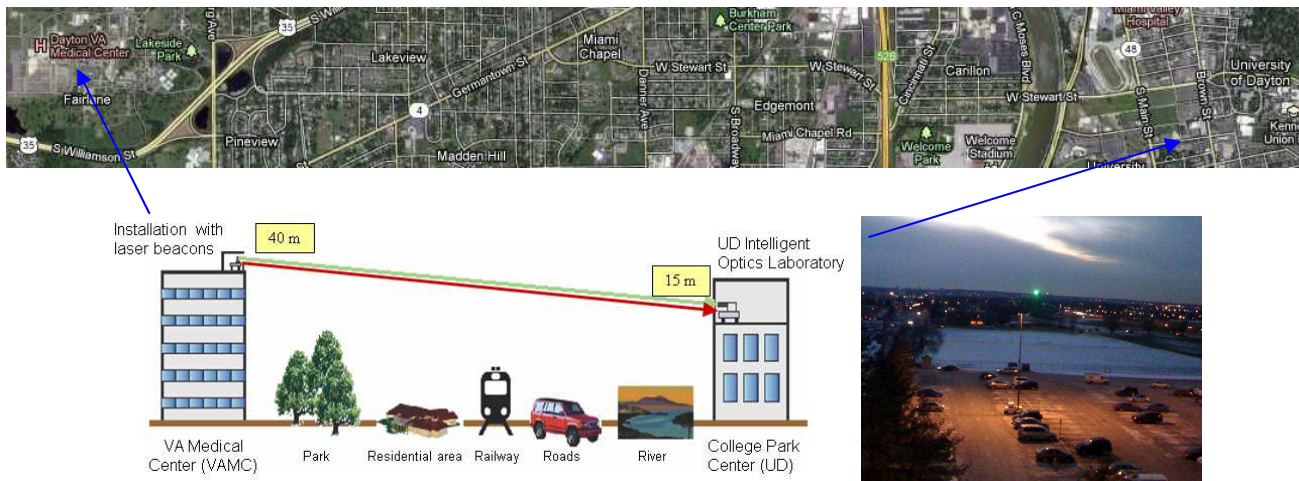
Figure 1. On top, an aerial view of the experimental site. Bottom, a graphical representation of the 7 km long atmospheric propagation path experimental setting (left) and snapshot of green laser beacon image taken from the receiver site at UD/IOL.
