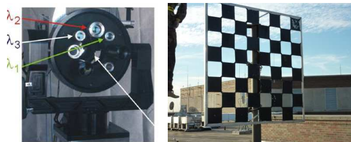
Figure 2. Left: the three laser beacons mounted on the gimbaled system; Right: the test pattern used for imaging applications.
