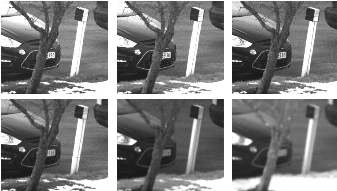
Figure 11. A small region of the scene as it was reconstructed in six band images. On the top row, from left to right, are the band images for 555-584nm, 584-613nm and 613-642nm. On the bottom row, from left to right, are the band images for 642-700nm, 700-758nm and 758-845nm.
