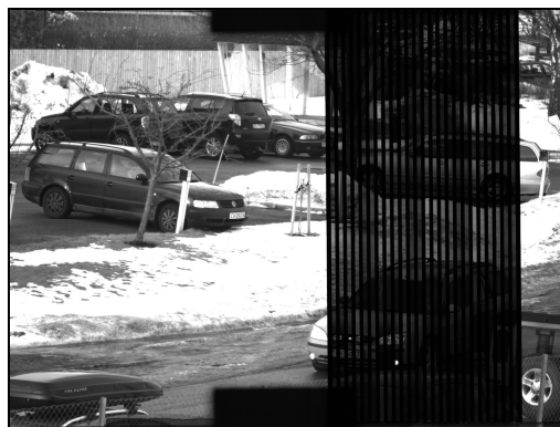
Figure 7. A single image from the demonstrator camera. The region with clearly visible vertical stripes is caused by the filter mounted directly in front of the detector array. The dark regions at the top and bottom of the image are due to the clamp holding the filter. The foreground car in the filter region is moving through the scene faster than the scan, potentially causing spectral artifacts.
