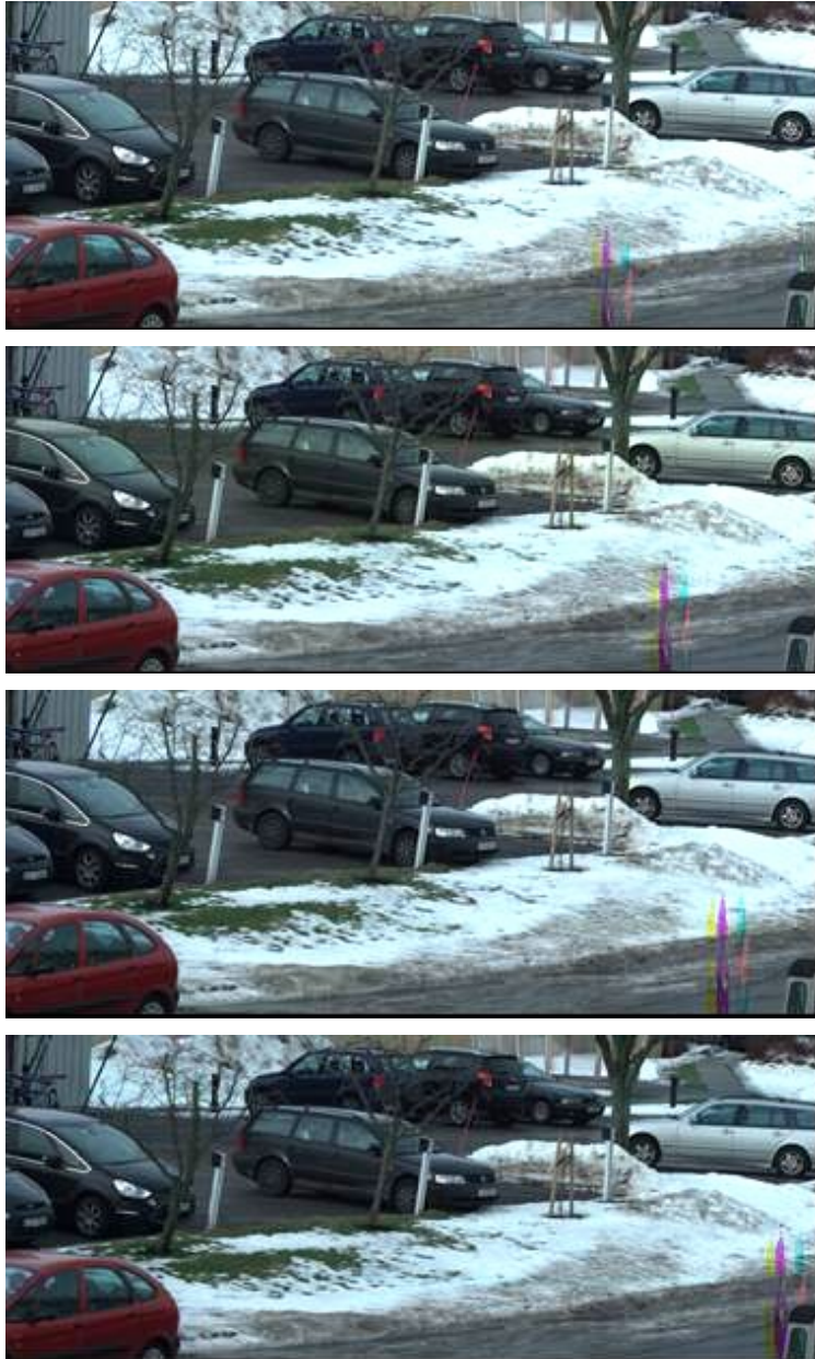
Figure 9. Four RGB images of the scene produced by combining spectral information from different filter stripes sampling the red, green and blue spectral bands. Spectral artifacts due to a passing car are clearly seen in the lower right part.
