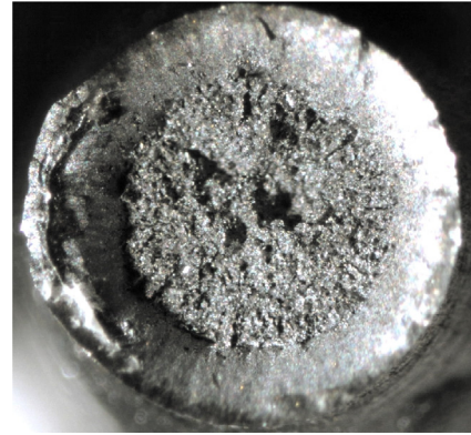
Fig. 3. The fracture surface of the smoothed bar.
