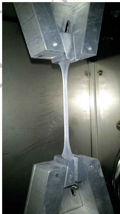
Figure 1. Tensile testing of dog bone-shaped, non-plasticized polymer samples (microtensile specimens according to ASTM D1708) using customized aluminium tensile grips. The picture is taken in the midst of an actual tensile test.
