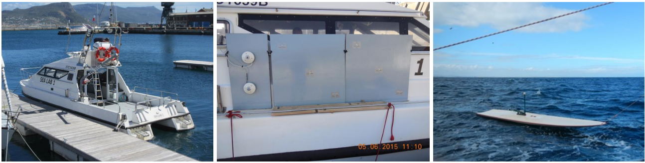
Figure 5: Research vessel 'Sea Lab 1', owned and operated by IMT (left). It served as primary asset during the intense observation periods. Middle: Steel plates used for dynamic signature/solar loading measurements. Right: Surfboard used for temperature profiles along the propagation path to Kalk Bay.
