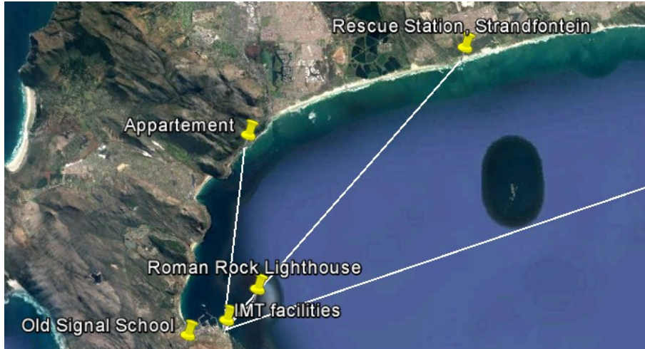
Figure 2: Positions of installations during the FESTER field trial. White lines indicate paths for propagation measurements during the trial (Image produced with Google Earth).
