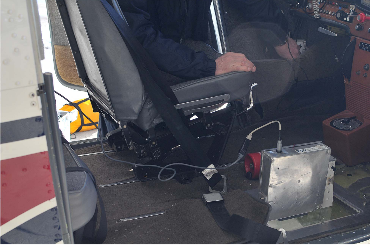
Fig. 5. Radar setup as seen through the passenger door of the aircraft. The gray aluminium box contains the radar, which is controlled from a laptop by the operator sitting at the rear of the plane. The hole on the floor is covered by a Plexiglass window, which has little attenuation for the radiated wave.
