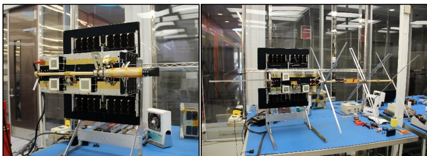
Fig. 1-12. Stowed (left) and deployed (right) VDES and AIS antennas onboard NorSat-2 in the SFL cleanroom.
