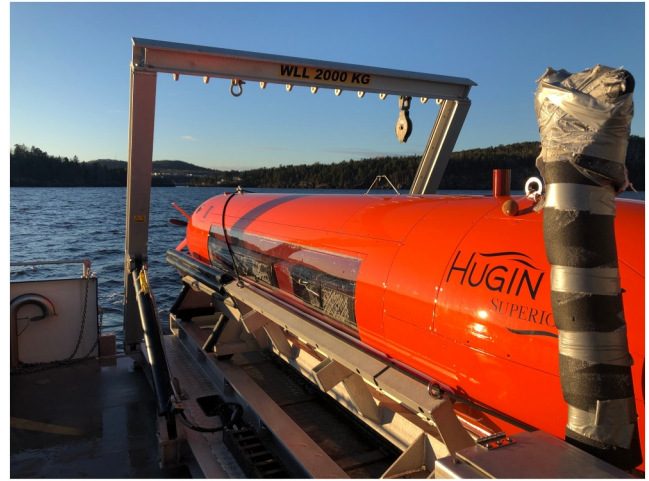
FIGURE 1 HUGIN Superior with the HISAS 1032 Dual Rx system. Photo courtesy of Kongsberg Discovery.
