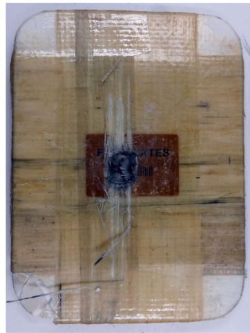
Target N, CP, 637 m/s. Front view of ceramic tile with filament-wound cover. (e)
