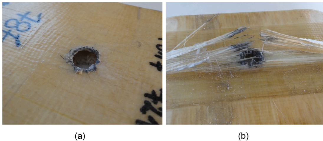
Fig. 9. Close-up of strike face and point of impact showing typical composite failure: (a) Little composite failure outside the point of impact in Target S (standard method). (b) Fibre delamination from the point of impact and towards the edge in Target N (new method).
