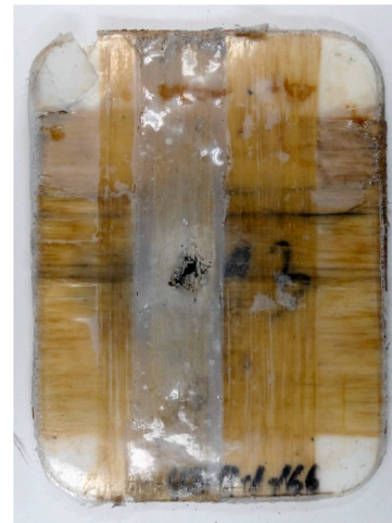
Target N, CP, 637 m/s. Back side of ceramic tile with filament-wound cover. (f)
