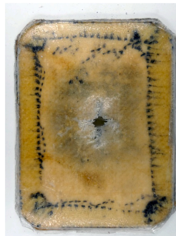
Target S, CP, 640 m/s. Back side of ceramic tile with fabric cover. (d)
