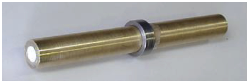
Fig. 2. The expanding ring test.
