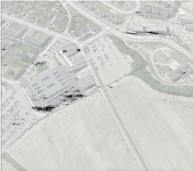
Figure 6. SAR dual-pol collection of area at Kjeller with the VERA system. SAR overlay in Google Earth. Buildings and lamp-posts is visible in the SAR image, amongst other features.
