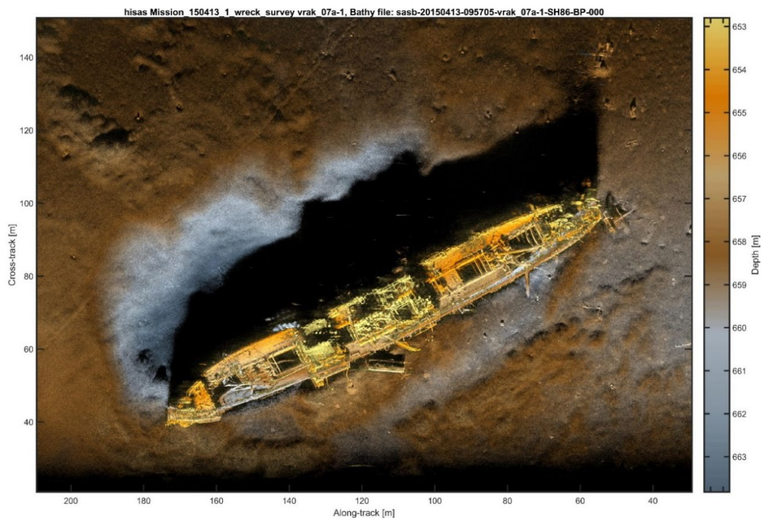
Figure 2.1 Fusion of SAS image and bathymetry of wreck 07 in the Skagerrak WWII dumpsite.
