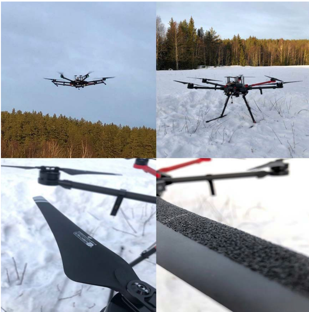
Figure 4.10 The DJI Matrice 600 during practical testing with emulated ice coating on propellers, January 2022. (Bottom left) Clean DJI propellers and (bottom right) propeller with emulated ice coating using an anti-slip tape. This ice emulation could roughly correspond to a moderate mixed ice buildup (FFI).
