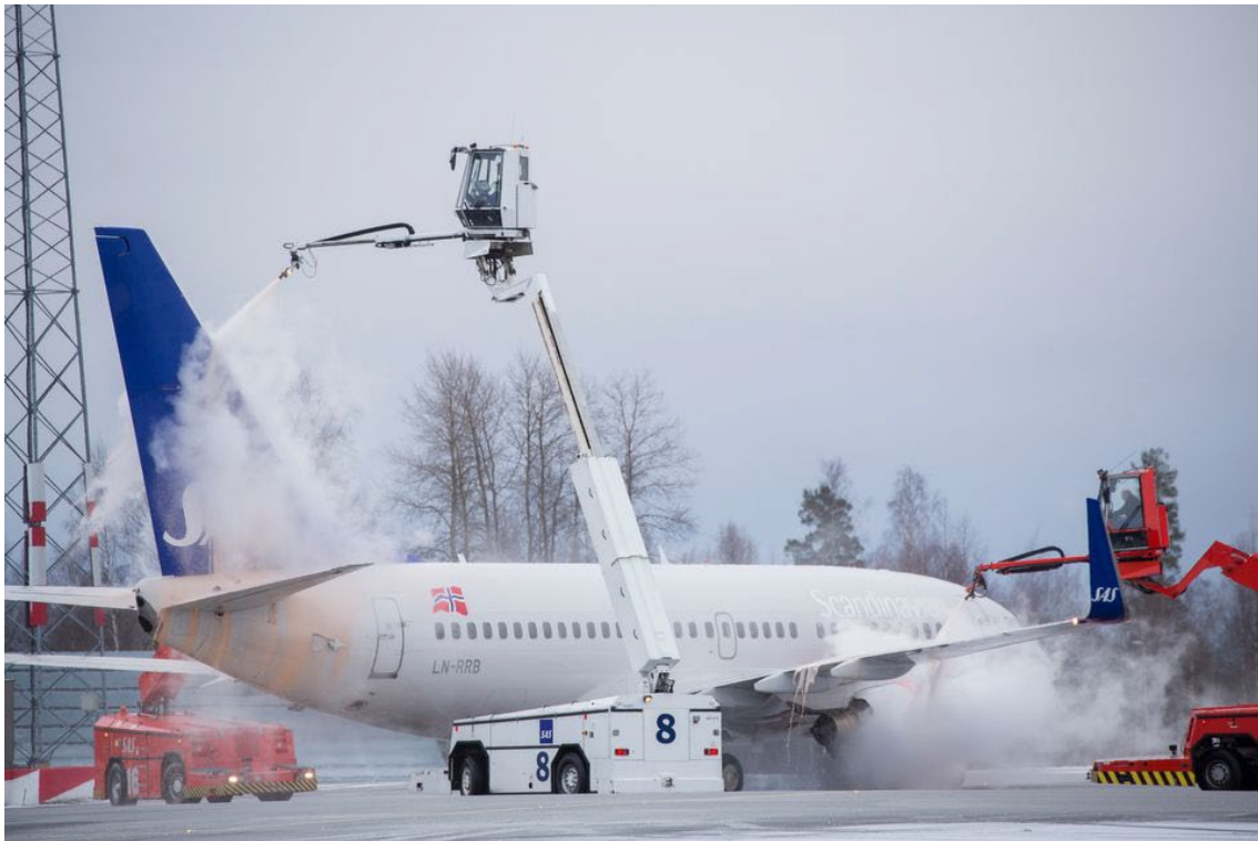
Figure 4.1 De-icing passenger aircraft is a costly and time-consuming activity, and critical to flight safety. The effect is temporary, so aircraft also depend on in-flight ice protection systems (IPS) to operate safely [20].
