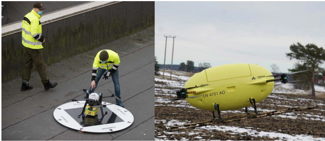
Figure 3.4 (Left) Senseloop with their drone developed by Globe, during testing from Rikshospitalet to Ullevål Sykehus in 2021 [16]. (Right) Sabrinus 4-20. Airlift Solutions tasked Sea Technology and Easy Form with developing this drone for use in their efforts in medical drone logistics. The drone has a 4kg internal payload capacity, 20 kg total weight and 20 km range [14, 15].
