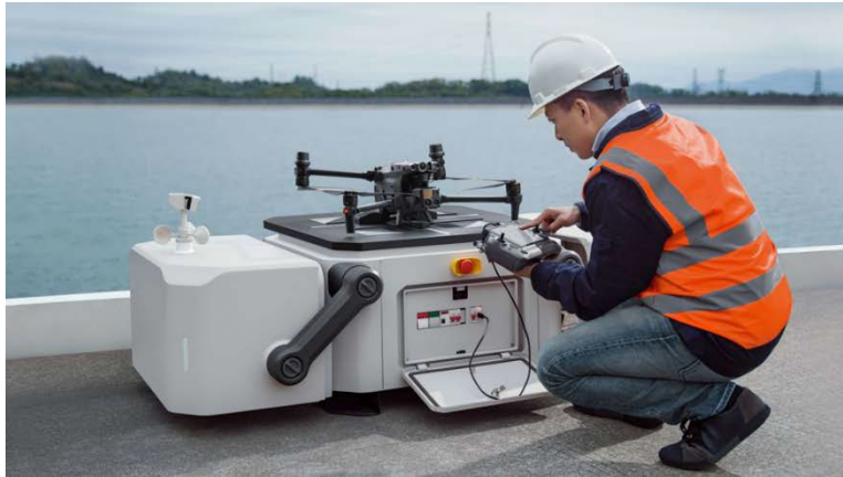
Figure 5.20 DJI has recently come up with a drone dock solution, which will allow remote controlled and automated operations [57].
