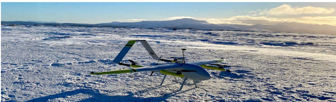
Figure 2.1 Norwegian company Aviant have performed a number of long distance winter flights as part of a push to realize medical logistics with drones. The aircraft and systems supporting them are not yet equipped for operations in icing or strong winds [13].
