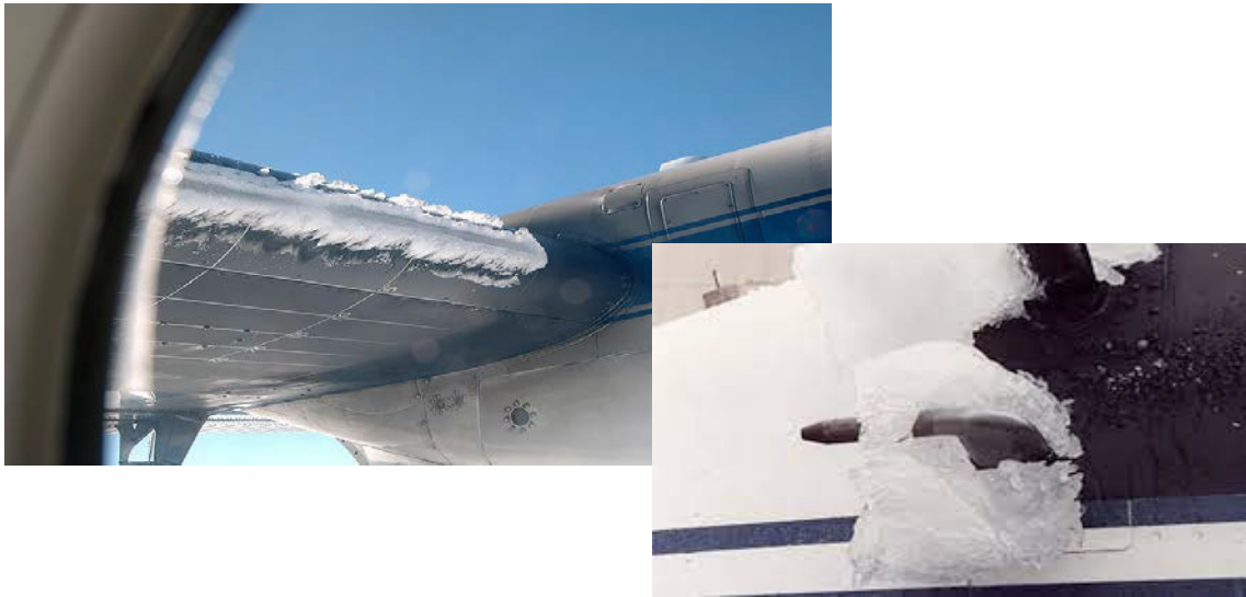
Figure 4.2 In flight icing on the leading edge of a NASA research aircraft (left) and an air speed sensor (right)[3].
