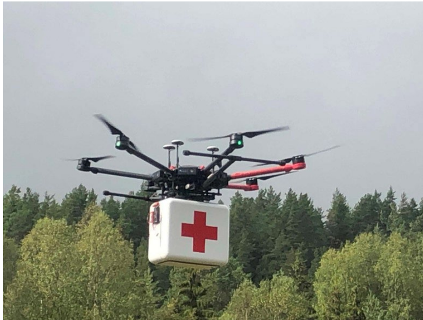
Figure 5.11 The DJI Matrice 600 is a typical professional drone, which we have used for practical tests. In this image, we have attached a payload section for testing purposes, which adds significantly to the drag and the moment of inertia of the aircraft. This is an example of “how not to do it”(FFI).
