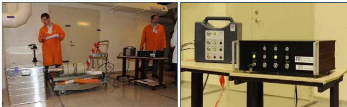
Figure 4.1 The information barrier system developed in the UK-Norway Initiative. The control unit gives a green light if fissile material is present and a red light if such material is not present. The pictures were taken at the Institute for Energy Technology in Norway during an exercise in June 2009.
