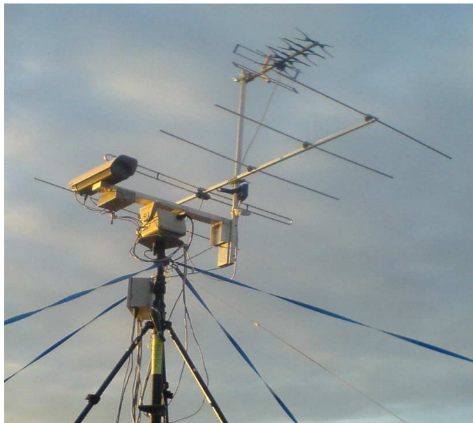
(b) Surveillance channel, DVB-T antenna; Funke Digital TV FFA4522 21/69 (upper antenna), FM radio; TRIAX 5 element (lower antenna).
