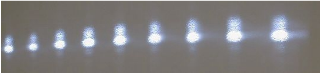
Figure 3.3 Photograph of the main and the side mode in the far field of the Coherent diode. The image of the laser diode was magnified in the x-direction by a 25 mm cylindrical lens
