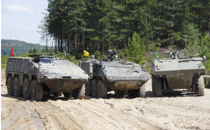
Figure 3.7 UK FRES candidates from left to right, ARTEC Boxer, Nexter VBCI and the GB Piranha Evolution [17]
