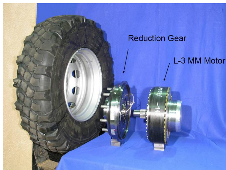
Figure 5.21 In-hub electric motor with reduction gear and wheel [24]
