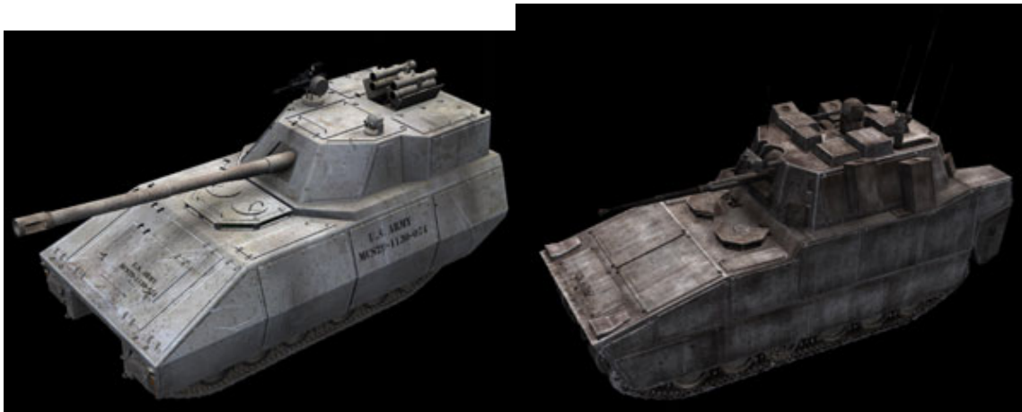
Figure 8.1 An artist's vision of the MGV Mounted Combat System (MCS) variant based on the GDLS chassis (left) and the Infantry Combat Vehicle (ICV) variant based on the BAE Systems chassis (right) [30]
