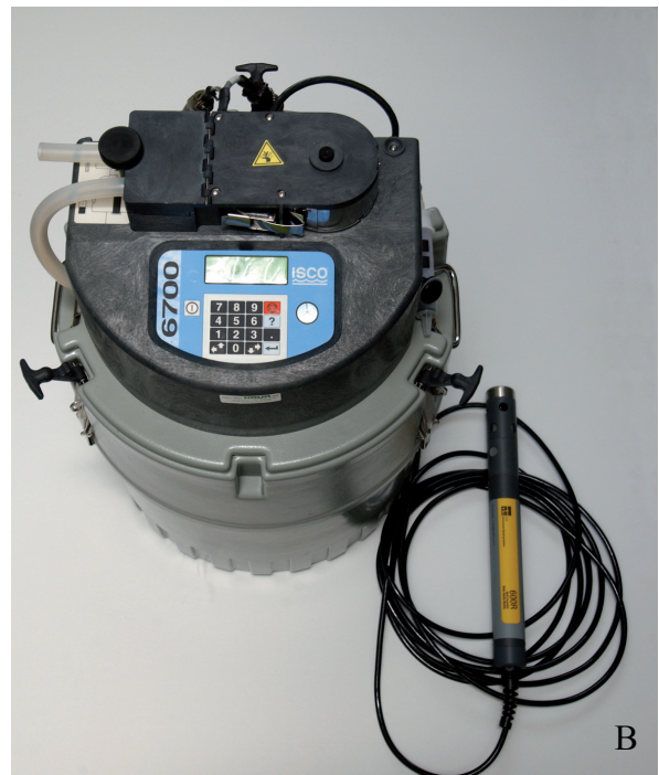
Figure 2.3. Custom-built transport container (A), containing fish tubs, power supply, automatic water sampler/logger (B: ISCO Model 6700 Portable sampler/Ysi multiprobe 600R) and facilities for in situ sampling (water fractionation, blood testing, organ sampling) and storage facilities. Photo: A E Strømseng.
