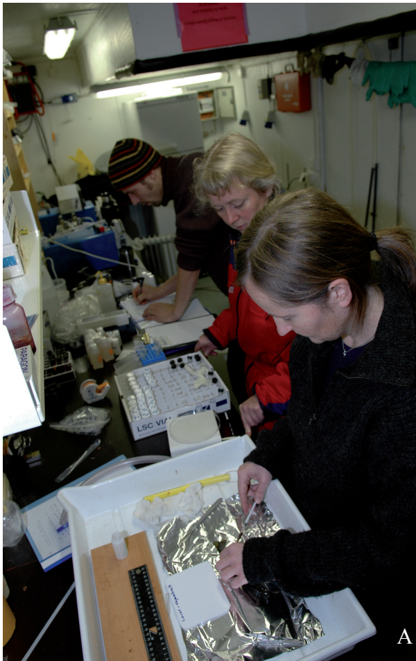
Figure 2.3. Custom-built transport container (A), containing fish tubs, power supply, automatic water sampler/logger (B: ISCO Model 6700 Portable sampler/Ysi multiprobe 600R) and facilities for in situ sampling (water fractionation, blood testing, organ sampling) and storage facilities. Photo: A E Strømseng.
