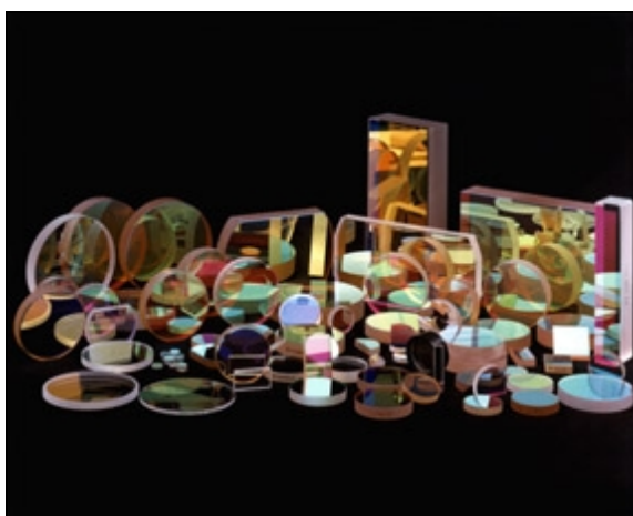
Figure 8.3 Photograph showing some of the approximately 4500 optical elements used in the AVLIS process. These high-quality optical elements reflect light approximately 100 times more efficiently than a bathroom mirror. Optical elements convey light through the laser system, and some also regulate the size and shape of the laser beams. Photo courtesy of the United States Department of Energy.
