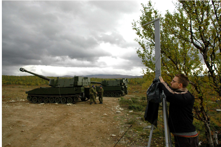
Figure 2.4: Emission measurements of M109, 155 mm field howitzer at Hjerkind.
