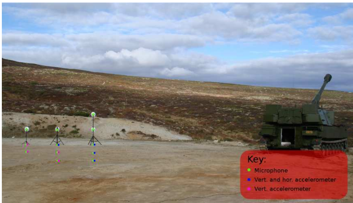
Figure 2.5: Near field measurement setup.
