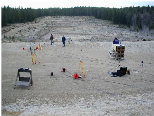
Figure 2.2: Emission measurements of small calibre weapons at Terningmoen.
