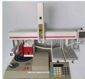
Fig. 4 Setup of the multipurpose autosampler for SPME and liquid injections (LOP): (A) hand-held-programming unit, (B) robotic head unit, (C) vial tray for SPME extraction, (D) liquid injection vial tray, (E) vial heater and agitation unit, (F) SPME fiber heater unit and (G) solvents for cleaning of liquid injection syringe. (Photo: Fremstad, FF)
