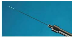
Fig. 1 SPME fiber coated with a polymer material (white needle tip). (Photo: Fremstad, FF)
