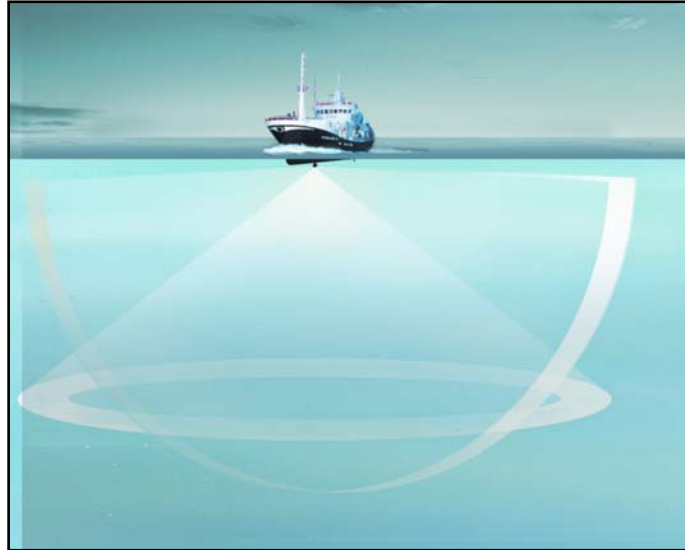
Figure 3.11. Illustration of horizontal and vertical sonar transmission from Simrad sonars.
