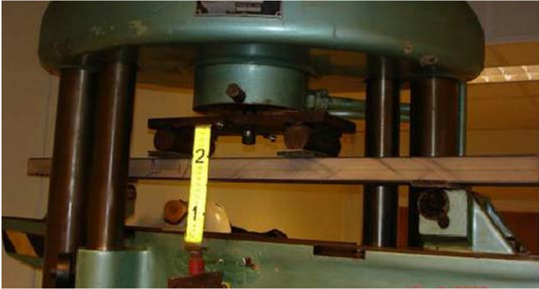
Picture 3.1 Test setup for ASTM C-393 4-point bending of sandwich beam
