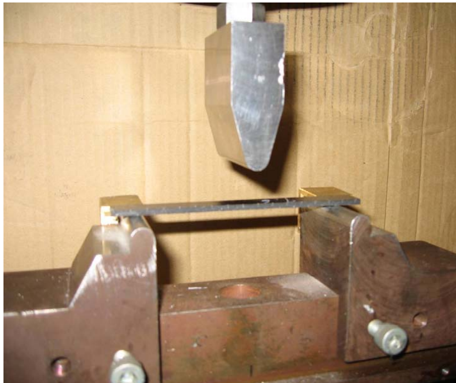
Picture 3.3 ASTM D 790 - Test setup.
