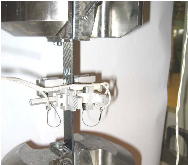
Picture 3.4 ASTM D 3039 - Test setup.
