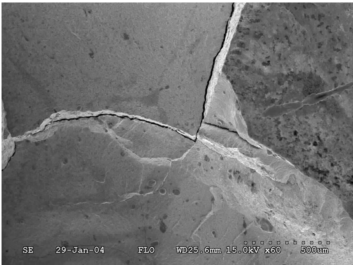
Figure 5.2: Fracture surface with cracks.
