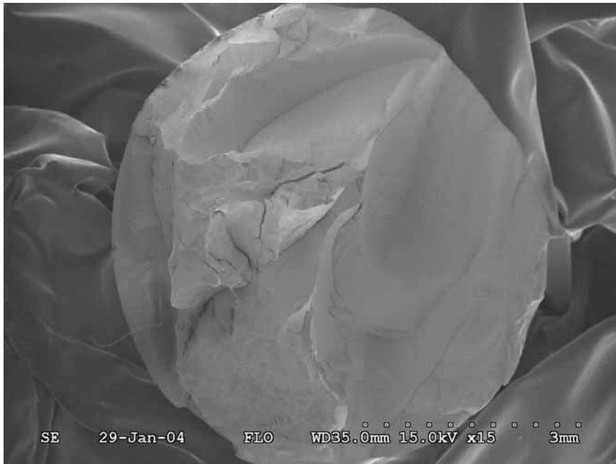
Figure 3.1: Overview of fracture surface (Sandvik Hard Materials)
