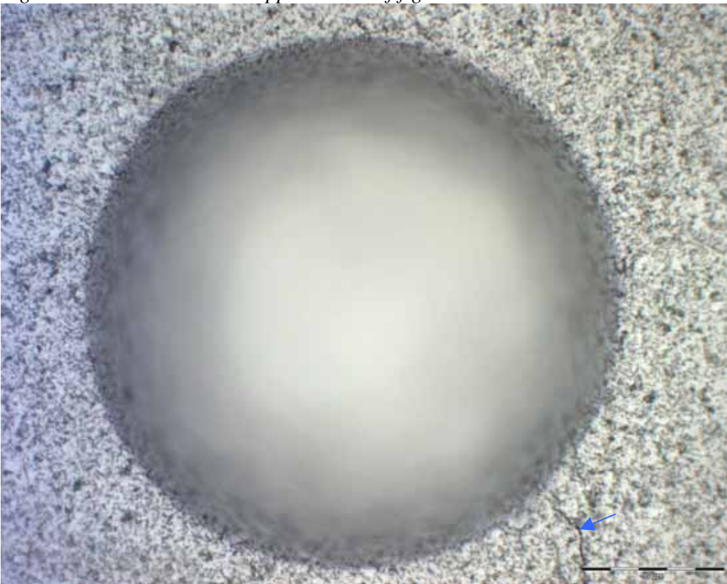
Figure 7.8: Hertel, Rockwell at 45 kg major load, crack emanating from the lower right edge.
