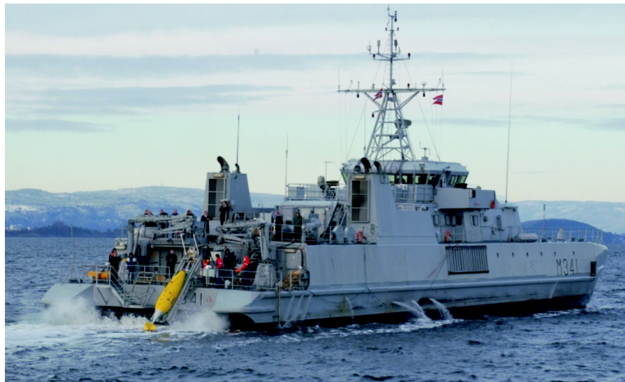
Figure 1.1 The HUGIN AUV immediately before launch at the RNoN mine hunter KNM Karmøy in December 2001.
