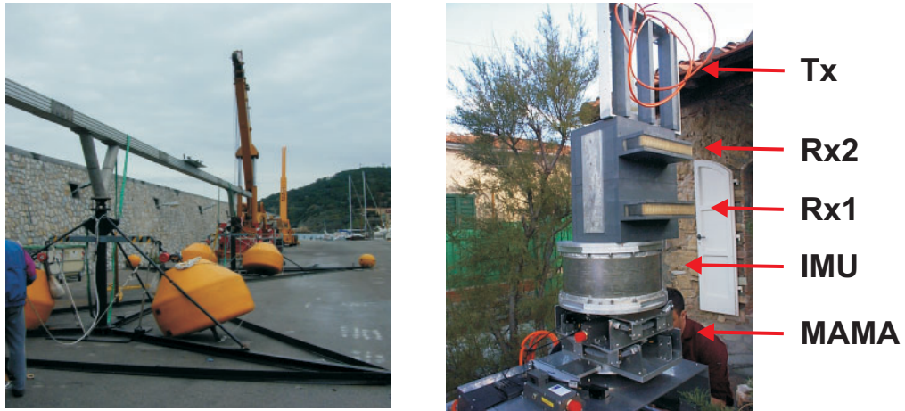
Figure 3.1 Left: Rail. Right: Sonar with IMU and MAMA.
