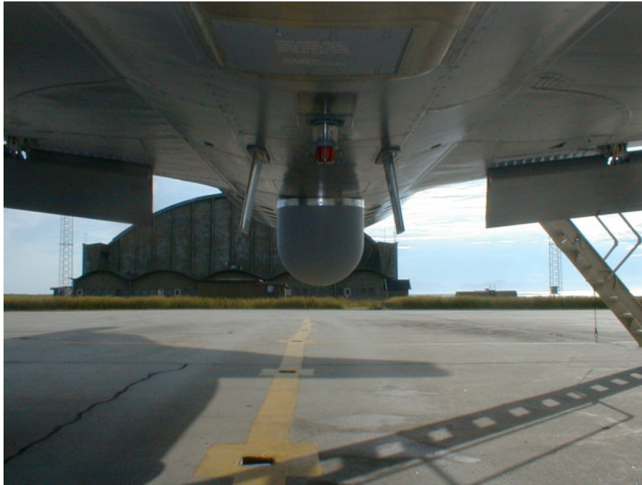
Figure 2.1: A backwards view of the radome under the airplane. Photo by Øistein Lundberg, FFI.
