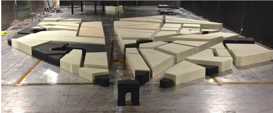
Figure 3.1 The Paris model inside the meteorological wind tunnel at the University of Surrey.
