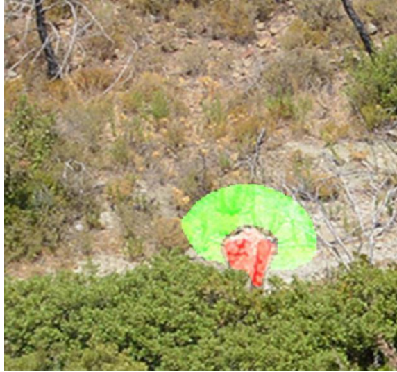
Figure 2.6 Illustration on how one of the targets was marked (red) in scene 2 for further use by CAMAELEON. The green halo above and to either side of the target shows one of our 5 differently chosen local backgrounds, to which the targets were to be compared, in order to find an estimate on the targets detectability, given in metres.
