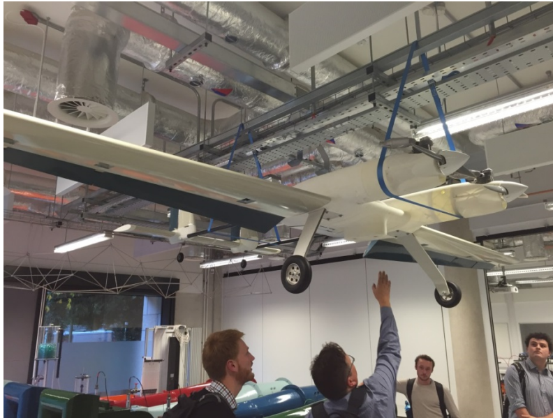
Figure B.1 The 2SEAS hybrid production UAV developed by the University of Southampton, UK. This is a low-cost UAV with wings from foam cutting technology and a 3D printed body. Flight endurance is 6 hours at 90 km/h with a payload capacity of 5 kg.
