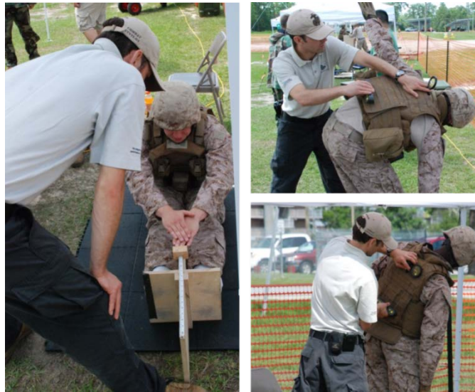
Figure 3.2 Range of motion measurements will be taken using a combination of a goniometer, a Wells and Dillon Sit and Reach apparatus, inclinometer, and a digital level.
